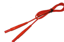
Test lead 1.2 m CAT III/1000V CAT IV/600V (2.5 mm 2 / banana plugs) red
